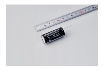
TOKYO, January 7, 2020 — TAIYO YUDEN CO., LTD. announced today the addition of LIC1840RH3R8107 ( $\phi$ 18 x 40 mm, 100 F) with an increased operating temperature limit of 105°C to its lineup of cylinder-type lithium ion capacitor LITHOSION<sup>TM \*1</sup> products.
